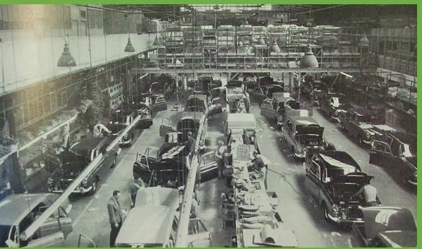
After 1968, the Daimler DS420 model was also built at Kingsbury, using pressed steel body panels brought down from Coventry.
